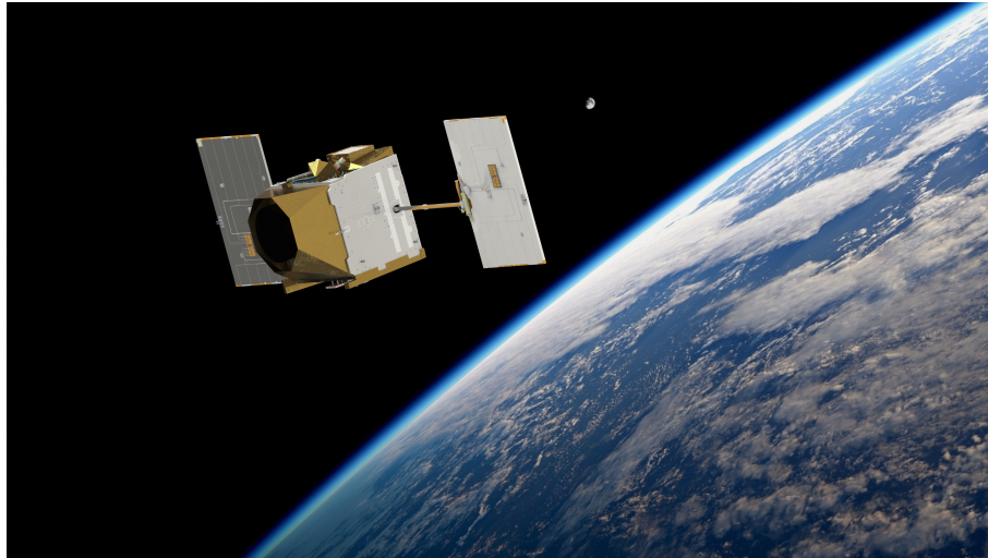
Figure 1: Artistic render of the Airbus Arrow platform configured for the Twinkle mission. Image credit: Airbus
